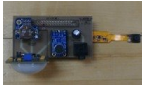
Fig. 2: Assembled sensor node.
