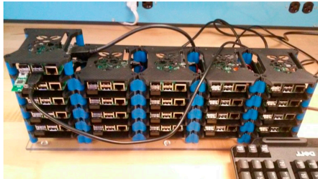
Figure 2: Final Raspberry Pi cluster.
